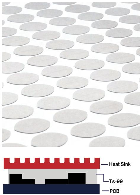
Ts-99 offers outstanding thermal conductivity at 24.0 W/m\*K and extremely low thermal resistance under minimal force. Ts-99 offers excellent compression, filling small air gaps on uneven surfaces, ensuring an efficient and consistent transfer of heat.
