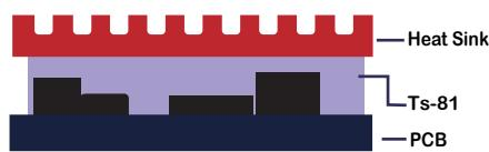
Ts-81 offers outstanding thermal conductivity at 8.0 W/m\*K and extremely low thermal resistance under minimal force. Ts-81 offers excellent compression, filling small air gaps on uneven surfaces, ensuring an efficient and consistent transfer of heat.
