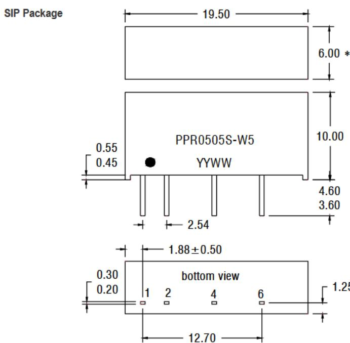
All dimensions in mm  $\pm 0.25$ mm. All pins on a 2.54mm pitch and within  $\pm 0.25$ mm of true position.
