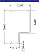
All dimensions in mm ±0.5mm. Tube length: 520mm Tube Quantity:15PCS
